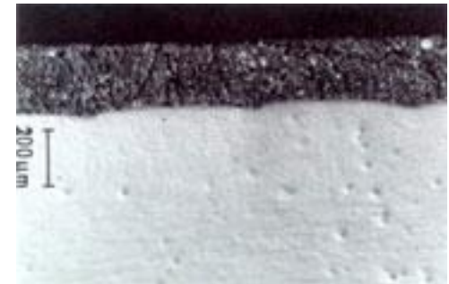
Cr 2 O 3 coating with a thickness of ca. 200 nm, deposited using a CO 2 laser and treated with a Nd-YAG laser.
